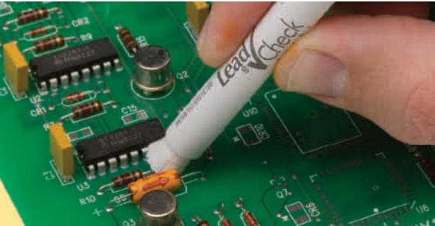
The test is totally self-contained! Just rub the solder joint or tinned component...
