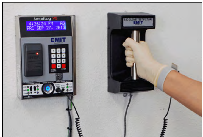
Figure 4. Using the ESD Glove Test Fixture with the SmartLog V5™
