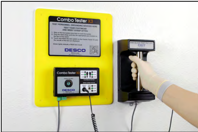
Figure 5. Using the ESD Glove Test Fixture with the Combo Tester X3
