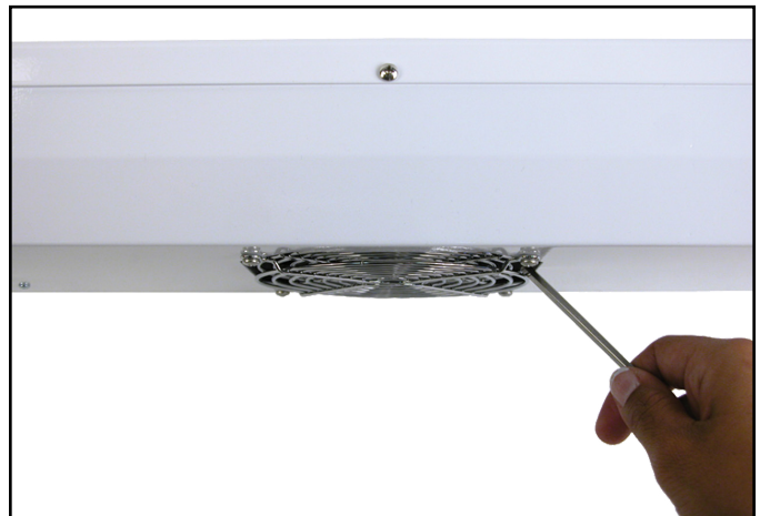
Figure 10. Shorting the ionizer’s two fan grills
